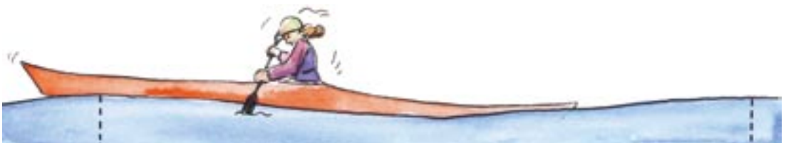
Fig 2.5c Sea kayak in a speed burst that can only be sustained for a short time. The bow is now lifting 5° off horizontal and the wavelength has increased to 18'. Speed is therefore 5.68 knots. Over very short distances some designs can exceed 'hull speed'.
