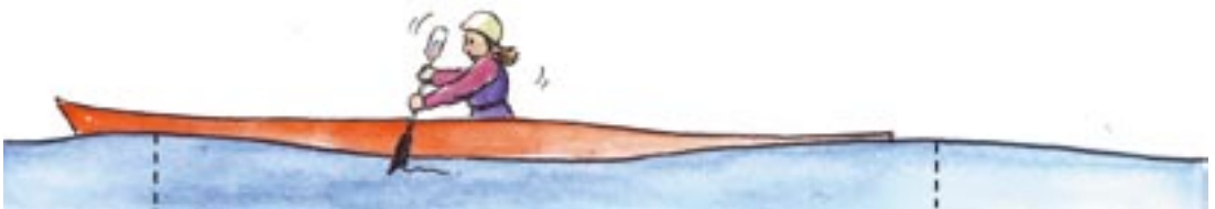
Fig 2.5b Sea kayak high speed cruising, wavelength almost the full waterline length of 14'. Speed is 5.02 knots. The kayak is starting to lift in the bow (2° off horizontal), and paddling effort is raised significantly.
