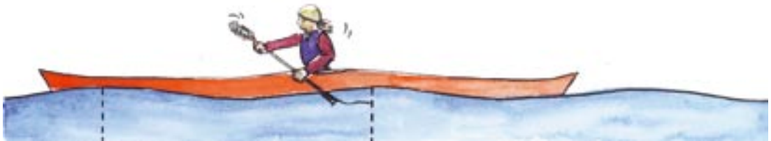
Fig 2.5a The theoretical max hull speed of a kayak with a 15' waterline length is \text{Speed (in knots)} = \text{square root of the waterline length} \times 1.34 . Therefore maximum theoretical hull speed is 5.19 knots.
