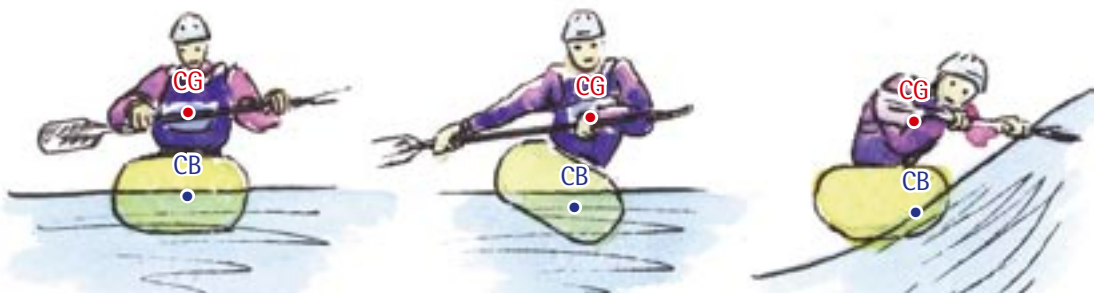
Fig 2.6a-c Figures a and b show a stable situation. C shows a paddler leaning into a wave to keep his CG over his CB, and using a bracing support to ensure he doesn't capsize.
